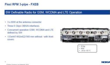
Gambar 3.5 Flexing RFM 3 pipe FXEB
