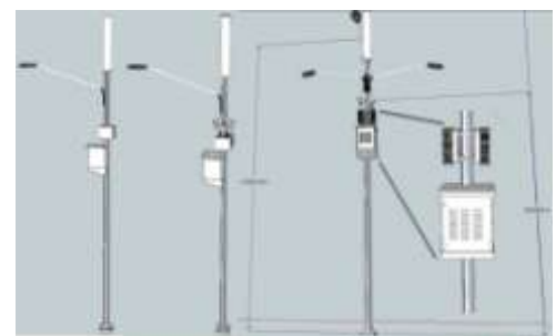
Gambar 4.8 desain BTS Hotel Pole
