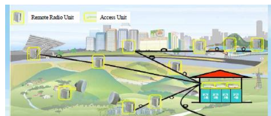
Gambar 2.1 BTS Room ke Pole
