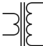
Gambar 2.7 Transformator step-up
