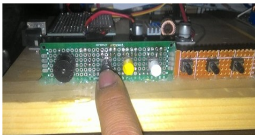
Gambar 12. Penekanan Push Button 1 (start)
