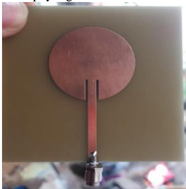
Gambar 4.1 Hasil design Antena mikrostrip
