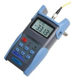
Gambar 3.2 Optical Power Meter sumber (Aprillia Sartika,2017)
